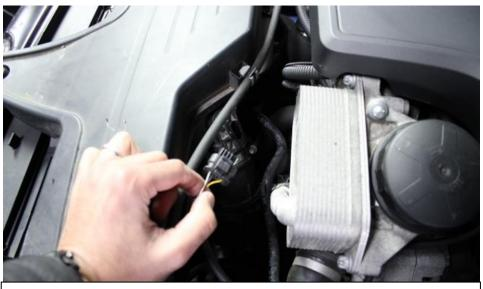
2. Remove the MAF sensor plug located at the back of the airbox.
