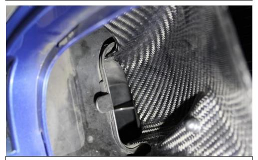
36. Move the scoop down so that the end of the scoop goes into the duct opening.
