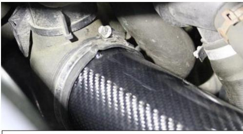
26. Push the carbon tube fully into the inlet hose – the notch on the carbon should go into the notch in the inlet hose. Secure the clamp around the hose.
