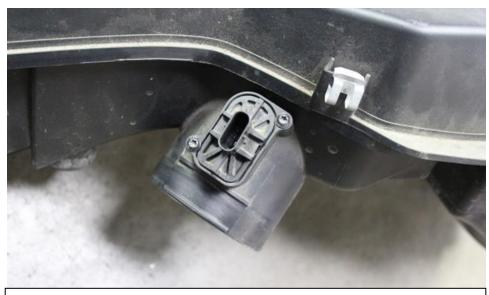
14. Remove the MAF sensor from the airbox – it is held in place with 2 torx screws.
