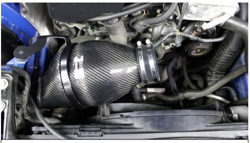
22. Push the supplied silicon coupler onto the filter housing with the 2 supplied hose clamps. Leave half the silicon extending outside the housing for the carbon tube. Secure the clamp around the Housing.
