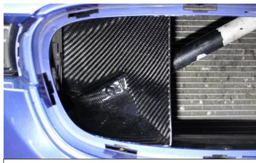
38. The lower panel of the scoop should line up behind the grill opening of the bumper.
