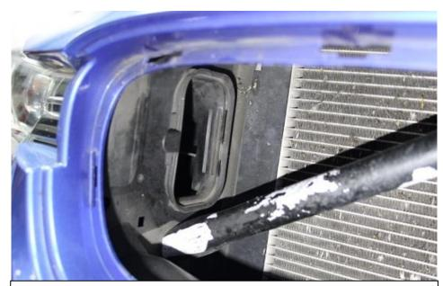
31. Remove the protective mesh inside the opening behind the grill. This is done by pulling the rubber tab and then taking the mesh out.
