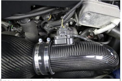
28. Firmly push the MAF sensor plug back into the sensor.
