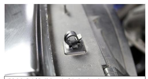
12. Push the clips in fully with the openings facing the engine as shown.
