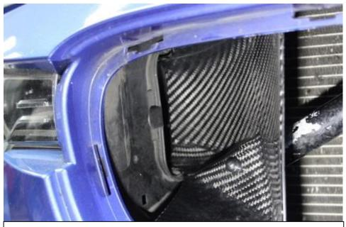
37. The end of the scoop should go inside the rubber duct opening.
