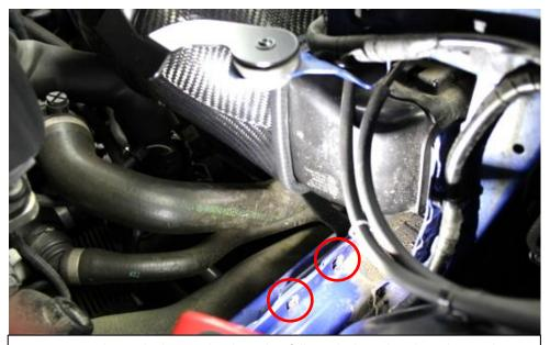
20. Here is another angle showing the plastic duct fully inside the carbon duct. There is also a bracket on the carbon duct which should line up with the 2 holes on the chassis as shown.
