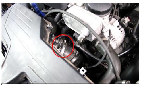
4. Loosen the hose clamp which secures the inlet pipe to the back of the airbox.
