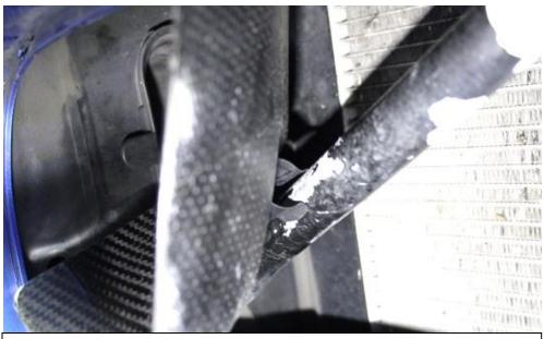
34. The clip should go over the strut bar.
