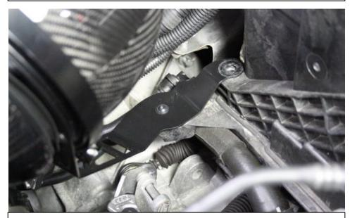
16. Once inserted the bracket should sit like this. Do not secure yet.
