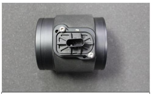
7. Insert the MF sensor into the new tube and secure with the 2 x supplied torx scews. DO NOT use the OEM screws for this. LCI version shown in next step.
