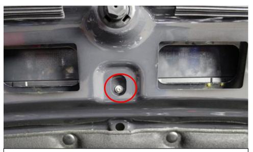
24. Now we will remove the bonnet scoop. Start by removing the torx screw shown.
