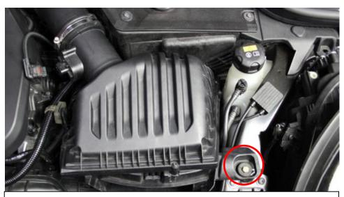
4. Loosen the hose clamp around the tube at the back of the airbox and remove the 10mm bolt as circled.
