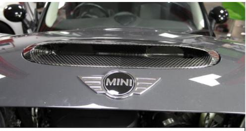
30. Once the clips are in position firmly push the scoop down in all 6 clip positions and ensure they click into place.
