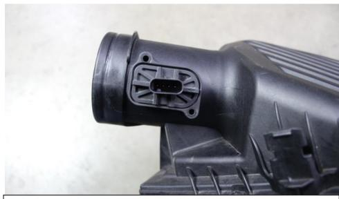
6. Remove MAF Sensor from the airbox by removing the 2 torx screws holding it in. The photo shows the pre-LCI version. The process is the same for the LCI model.
