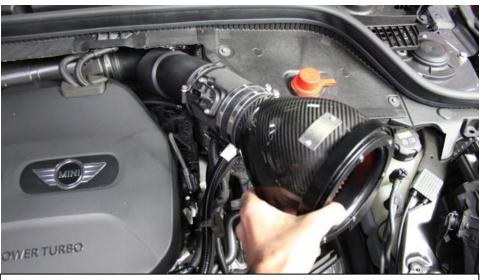
14. Push the filter housing and MAF tube into the stock intake tube.
