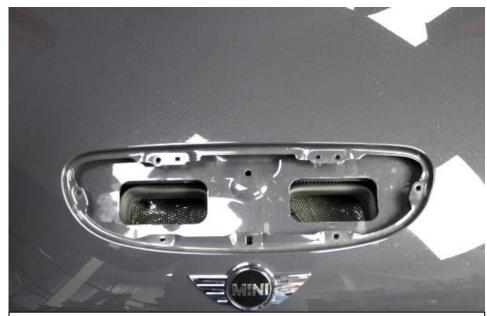
27. With the scoop removed – the clip locations can be seen on the bonnet ready for the carbon scoop.
