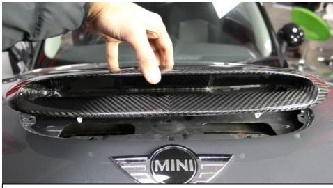
29. Carefully lower the carbon scoop into position – make sure the 6 clips are already installed on the back of the scoop.
