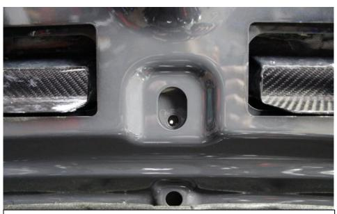
31. Once clipped into place – secure the scoop by screwing the torx screw removed in step 24. IF your scoop came pre-assembled with a new screw in this position from step 28 – use the new screw to secure the scoop.
