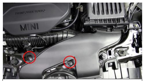
1. We will start by removing the intake duct. Remove the 2 x 10mm nuts as circled.
