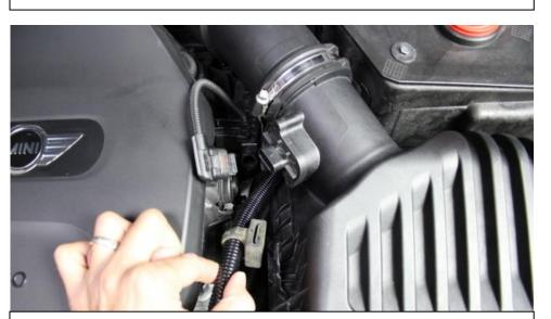
3. Disconnect the MAF sensor and remove the rubber holder from the airbox.
