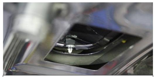
25. The scoop is held in place by 6 clips. You can compress the ends of the clips which are accessible and lift the scoop out. The next photo shows the back of the removed scoop and the locations of the clips.
