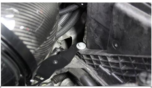
18. Once the duct and housing are aligned – secure the bracket with the bolt removed in step 5.
