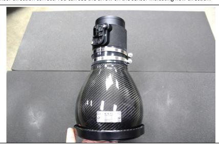
11. Rotate the MAF tube so that it is positioned as shown relative to the Eventuri Badge on the housing. Tighten the hose clamp around the filter housing. Leave the other one loose for now.
