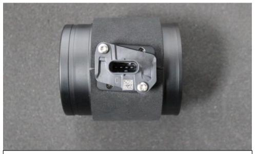
8. Here is the LCI version of the MAF tube and sensor – secure with the new supplied screws.
