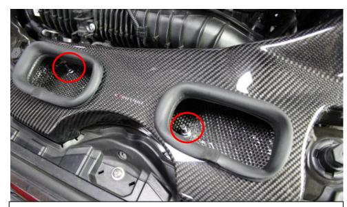
20. Now secure the duct with the 2 x M6 nuts.
