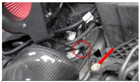
15. At the base of the bracket on the housing there is a mounting locator (circled) – push this into the rubber grommet indicated by the arrow. You will need to lift the duct to allow the filter housing to be lowered into place.
