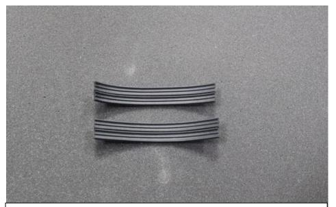
21. Take the 2 rubber strips provided. These will protect the carbon duct against the bonnet.
