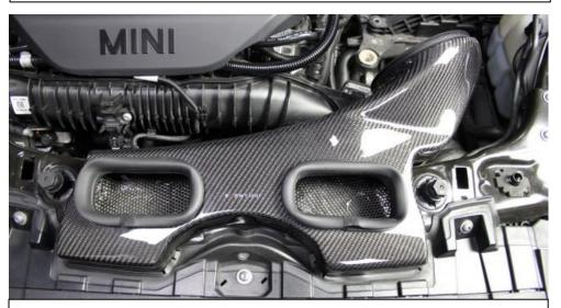
12. Insert the carbon duct into place – the 2 threaded studs should go through the holes in the base of the duct – see the next photos.
