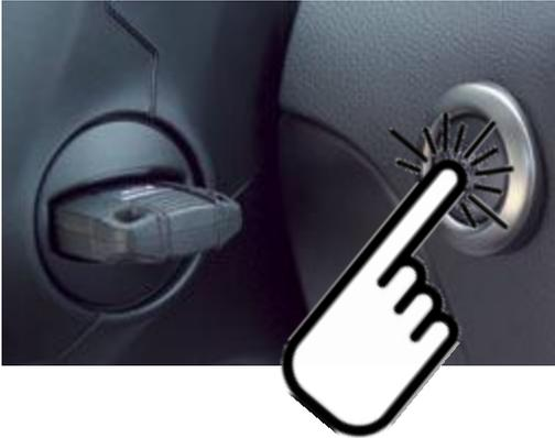
To switch on your ignition inserting the key is not enough, you have to push the start button once as well. Without pushing any pedal.
